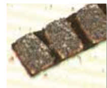
2D+3D Image with clear low bridge defect
